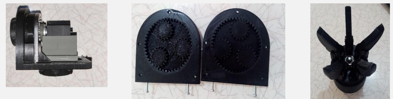
Figure 3: 2 DoF Spherical Manipulator Proposed for the Orientation System
