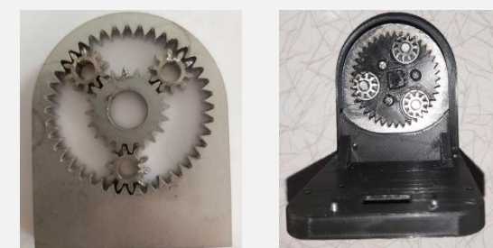
Figure 4: Planetary Gear with 1:3 Gear Ratio Produced by Sheet Material
