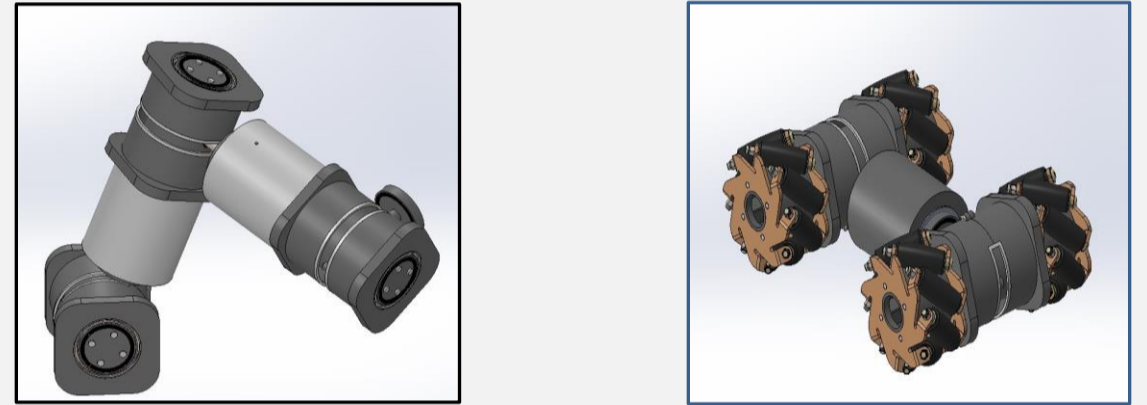
Figure 3: Serial Arm and Mobile Manipulator Configurations
